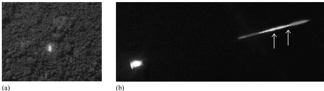
Figure 4 LIBS plasma formed on ordinary soil
